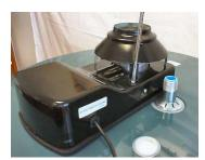
With a #2 Philips, remove the damper cover retainer screws. Gently lift the damper cover from the water heater.
