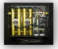
Here is a look inside the RTE-27 product. Notice there are four heating elements (tubes) that are used to heat the water. Also notice there are two field wiring connections at the bottom right of the unit. Each of these wiring connections needs its own 60 amp breaker for a total of 120 amps.
