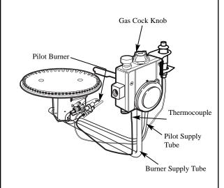
Replace main burner natural gas orifice with the Red colored main burner orifice (stamped LP) supplied in the cloth bag. Refer to the Replacement parts section in this manual for the location of the orifice on the burner assembly.
