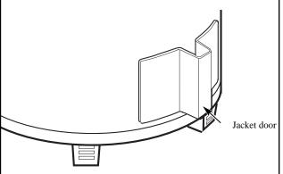
NOTE: Make sure tabs on inner door engage inside the opening of the inner skirt.
