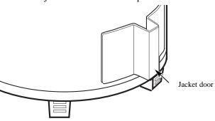
NOTICE: Make sure tabs on inner door engage inside the opening of the inner skirt.
