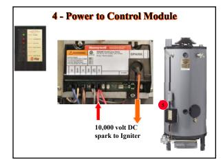
Power is now being supplied to the 24V terminal of the control module by the red wire. This is the only wire that feeds power to the control module.
