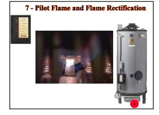
The pilot gas is ignited by the sparking pilot electrode and the pilot flame is established.
