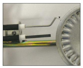
Y positioning (side view distance from top of burner plate)
