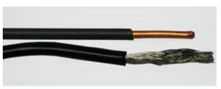
2. Put wires together and wrap the stranded wire around the solid.
