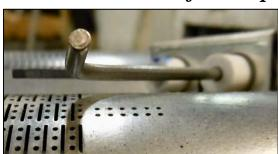
Flame rod should be positioned as shown.
