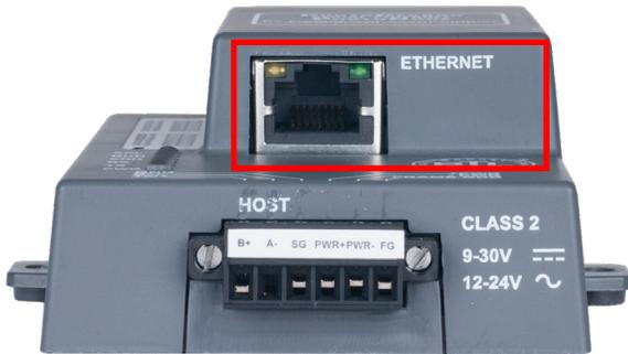
Figure 12. Ethernet port location of ProtoNode
