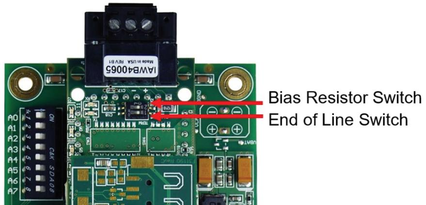
Figure 9. End-of-line termination on from ProtoNode to RS-485 Field Protocol – BACnet MS/TP
