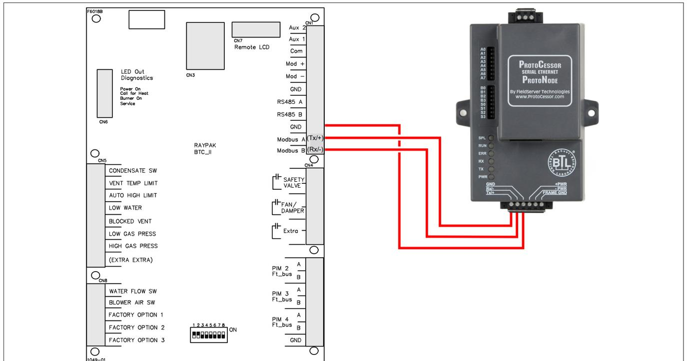
Figure 6. VERSA IC Modbus RS485 pin outs to the ProtoNode's Modbus port
