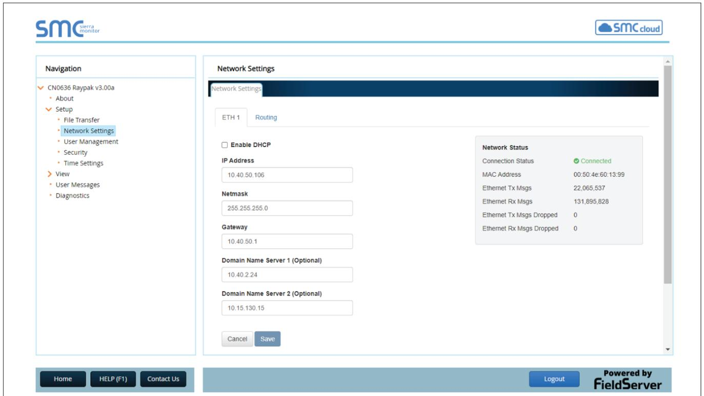
Figure 18. ProtoNode Network Settings Tab
