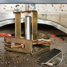
Look inside the combustion chamber and locate the TRD housing. It is in the middle of the combustion chamber.
