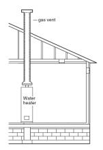
Single appliance venting is the traditional method of one vent pipe per water heater.  $\leftarrow$
