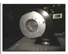
Don't forget to clean the inlet air screen on the blower. If it becomes clogged, you will get a pressure switch error code.
