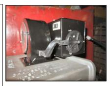
120V power is passed from the control – to the black wire – and to the blower motor. This black wire is the only source of AC power for the blower motor.
