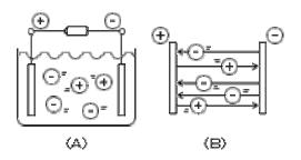
When a voltage is applied, the ions move straight toward the respective oppositely charged metal plates, as illustrated in Fig. (B). (<u>http://global.horiba.com/story\_e/conductivity/conductivity\_04.htm</u>)
