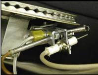
5. Remove the thermocouple from the burner assembly by pulling it thru the orange plug. Pull from the outside of the inner door. (Removal is easier if you cut the thermocouple with wire cutters.)
