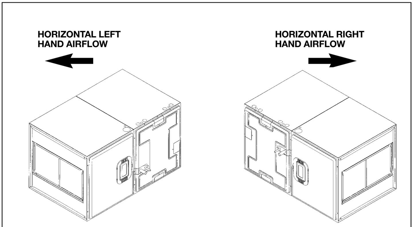
**NOTE:** Coil and blower section are always in a draw through configuration.
