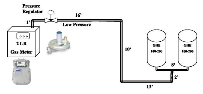
High-pressure side is no problem. We carry 2 psi to the pressure regulator. The pressure regulator reduces the pressure to the rating specified on the rating plate. In this case, it is 10" w.c. natural gas. Then we have 49 feet of pipe from the regulator to the water heaters. The water heater input rating is 400,000 BTU for both heaters. If you check the pipe-sizing chart, the pipe size from the pressure regulator to the water heaters is 1 ½ inch minimum.
