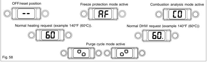
**NOTICE:** When the request for heating and/or hot water has been satisfied, the boiler pump and fan may continue to circulate to dissipate any residual heat within the boiler.
