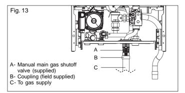
**NOTICE:** When installing the gas supply connection, it must comply with local regulations or, if such regulations do not exist, with the National Fuel Gas Code, ANSI Z 223.1.
