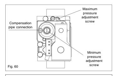
**NOTE:** The gas valve sticker "WARNING: VALVE IS NOT FIELD SERVICEABLE" means the valve can be adjusted but not disassembled.
