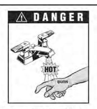
Water temperature over 125°F - 50°C can cause instant severe burns or death from scalds.
