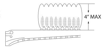
Fig. 2: Correct Main Burner Flame Pattern
