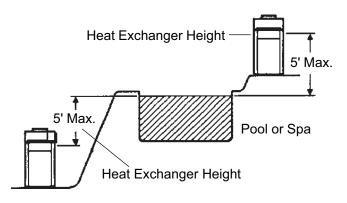
Fig. 25: Above/Below Installation Limits
