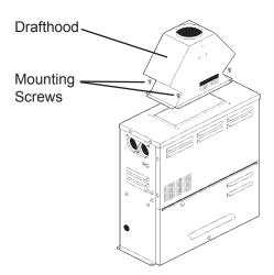
Fig. 8: Heater with Indoor Top
