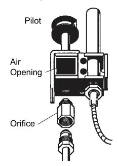
Fig. 28: Honeywell Pilot
