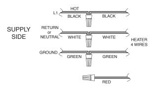
Fig. 20: 120V Wiring
