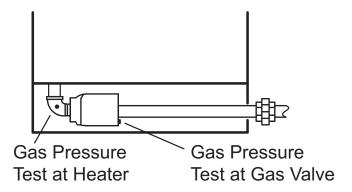
Fig. 11: Gas Pressure Testing Locations
