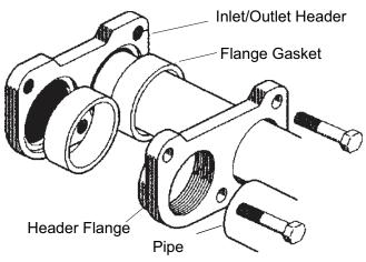
Fig. 15: Header Connections
