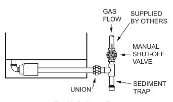
Fig. 10: Sediment Trap
