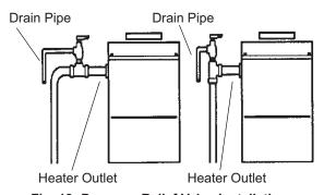
Fig. 18: Pressure Relief Valve Installation
