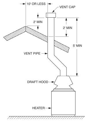
Fig. 9: Venting Clearances
