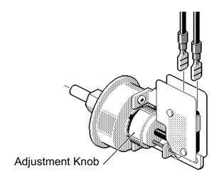
Fig. 24: Pressure Switch Adjustment
