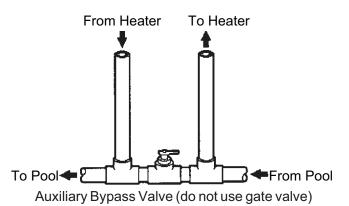
Fig. 17: Auxiliary Bypass Valve
