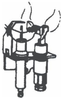
Fig. 2: Pilot Burner Flame
