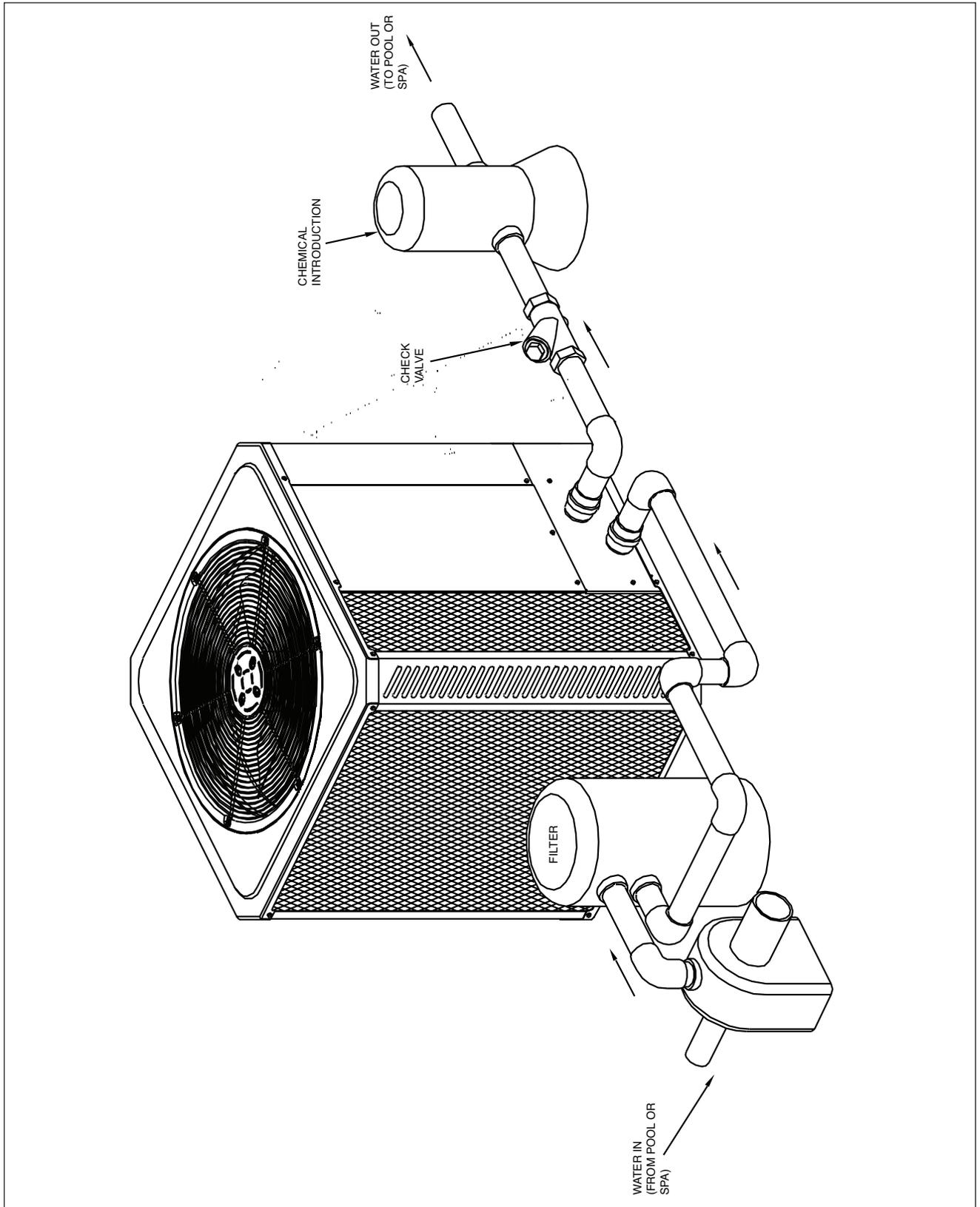
**Fig. 6: For systems with pumps of less than 2 HP (under 80 gpm), no external bypass is required. Connections are 2-inch unions. Plumb the heat pump pool heater AFTER the filter and BEFORE any chlorinators.**
