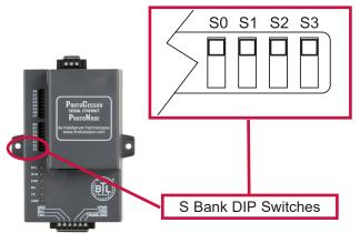
Figure 2. S0 through S3 DIP Switches
