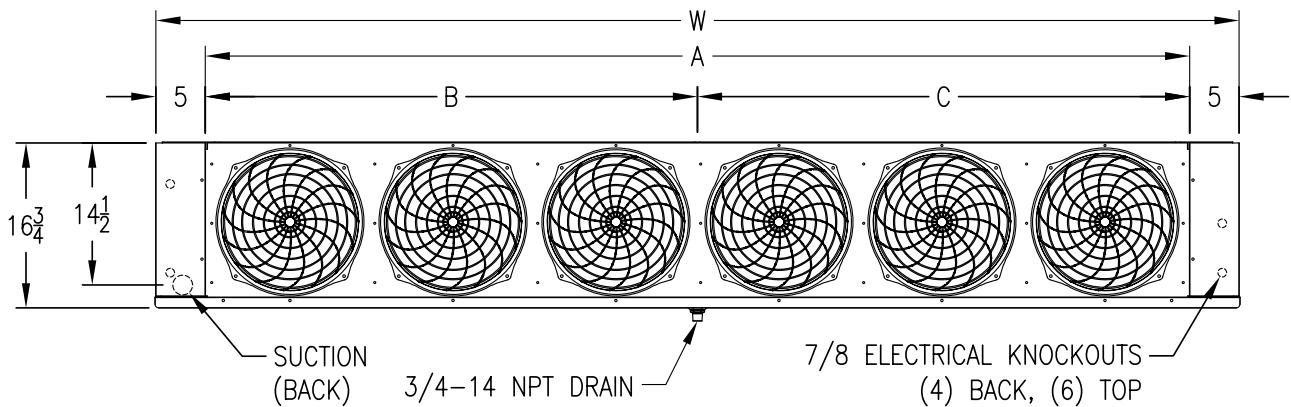
**NOTE:** Refrigerant and electrical connection locations have been changed for the Next-Gen All-Temp design. Standard connections are now opposite of the legacy All-Temp models.
