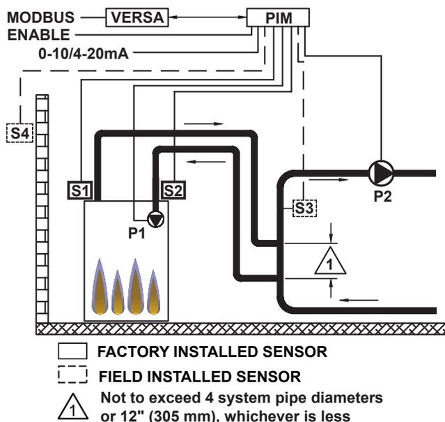
**Figure 16. Mode 1 - Single Boiler with Primary/Secondary Piping**
