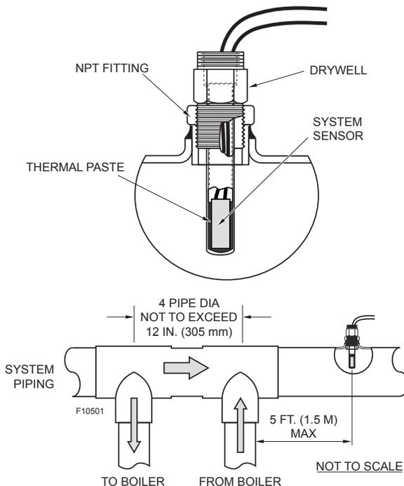
Figure 13. System Sensor Installation
