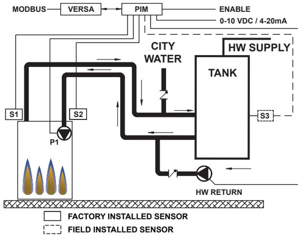
**Figure 20. WH Units - Single Water Heater with Tank
