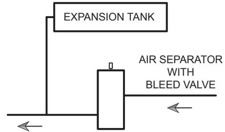
**Figure 14. Air-Separation/Expansion Tank**
