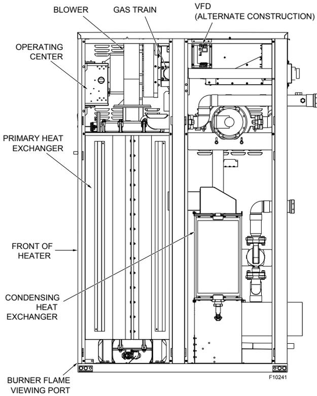
Figure 1. Component Locations – Side View
