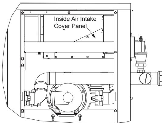
**Figure 8. Install the Inside Air Intake Cover Panel**
