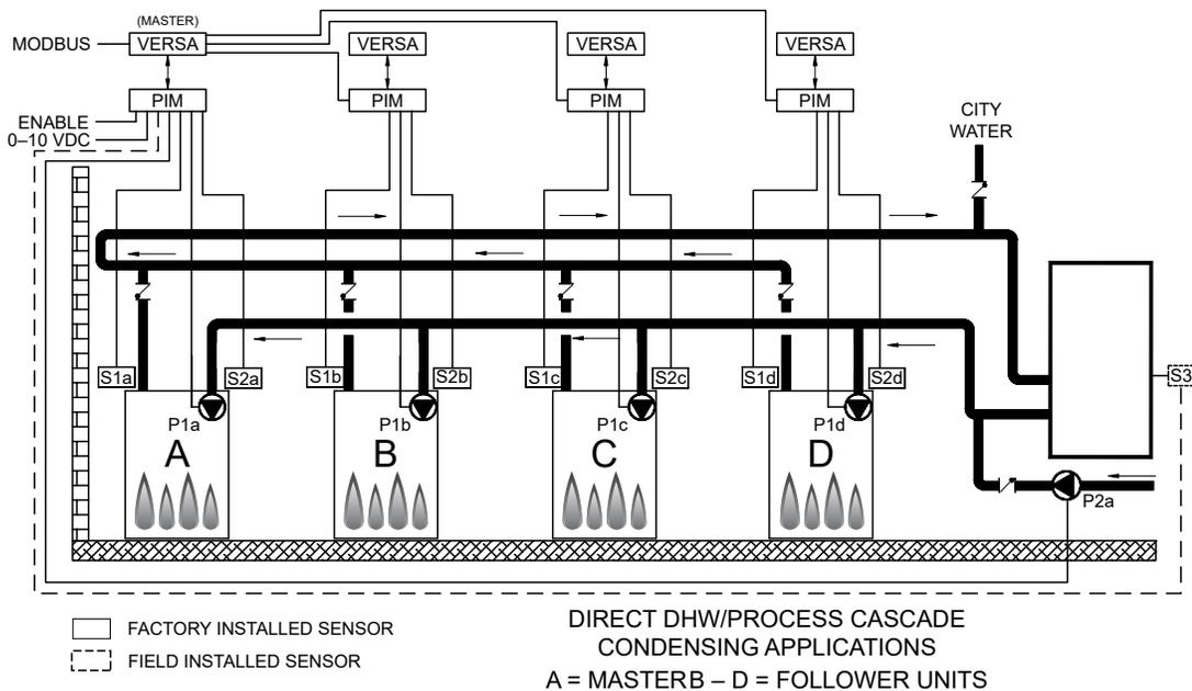
**Figure 21. WH Units – Water Heater Cascade with Tank
