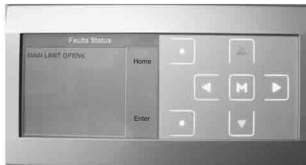
FIGURE 104 FAULT MESSAGE (IF ANY) ( MAIN LIMIT OPEN ) DISPLAYED.
