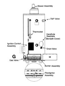
properly adjusted for operation on natural gas with a stainless steel burner. Water Heater shall have a spark-to-pilot ignition system. Controls will be arranged for safety shutoff in event of pilot failure. Complete unit shall be insulated with fiberglass insulation. Water Heater shall be covered by a three year limited warranty against tank leaks.
