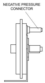
Figure 6. Draft Proving Switch
