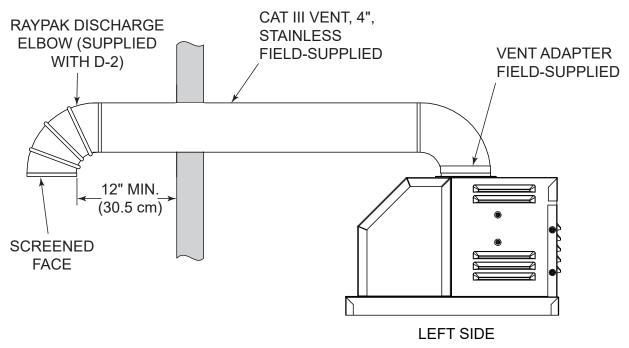
Note: The 90° elbow must be used as the termination cap.
