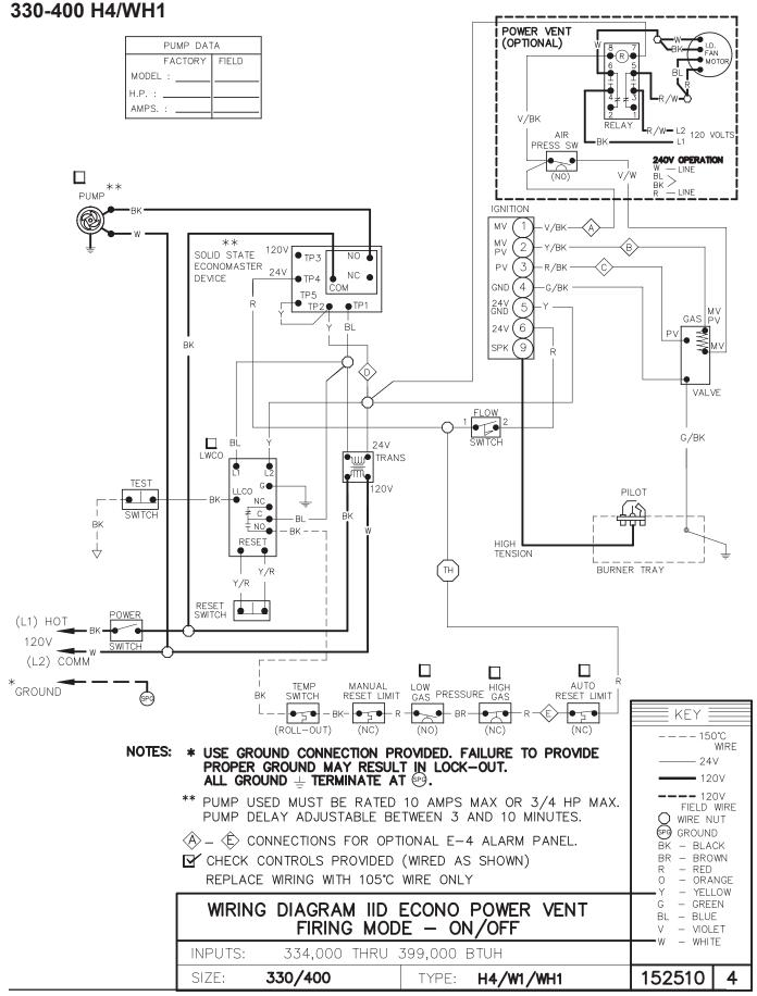
Note: Use the wiring diagram provided with the heater.
