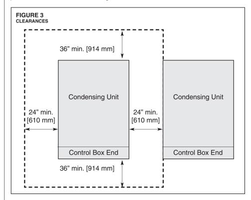
The unit must not be connected to any duct work. Do not locate unit under a roof drip; if necessary, install gutters, etc., to prevent water run-off from hitting the unit. To prevent air recirculation, it is recommended that the unit not be installed under an overhang, but if necessary allow a minimum of 60 inches above the unit for air discharge.
