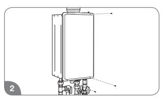
Remove the front cover panel on the water heater.
