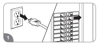
Ensure that the power to the water heater has been disconnected.
