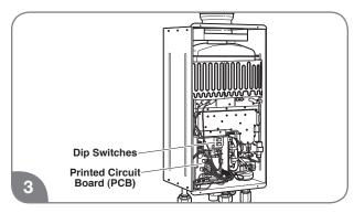
Find DIP Switch 2 located in the top-right portion of the PCB. The switch labeled "DIP 2" is the bottom switch.
