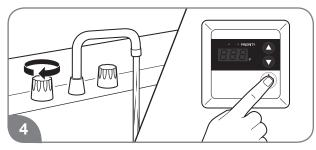
Turn on a hot water faucet and recheck the remote control display.
