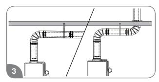
Support vertical and horizontal runs as described on page 36. Vertical supports are required every 4 ft. (1.2 m) along a vertical pipe route, after every transition to vertical, and after every offset elbow.
