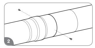
Attach the female end of the next vent pipe section to the male end of the 3-in./5-in. (7.6-cm/12.7-cm) concentric vent pipe. Push firmly on the pipe until the outer jacket has made contact with the snap ring on the male end of the concentric vent pipe section. Secure the two pipe sections with the provided self-tapping screws.
