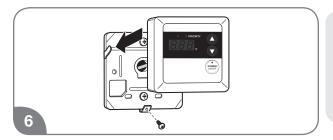
Position the remote control on the base plate.
