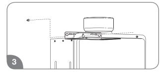
Position the upper mounting bracket and partially install the center mounting screw. The clearance between the screw head and the wall should be about 1/8 in. (0.3 cm). Hang the upper bracket on the screw.
