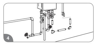
Using the proper-size piping, fittings, and components, build the gas supply line to the water heater.
