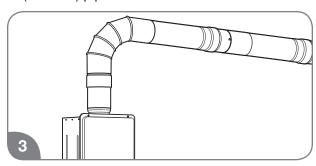
Attach required vent sections between the water heater collar and the horizontal vent termination.
