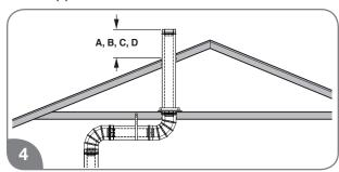
Determine the vent terminal height and install the vent pipe accordingly. Refer to "Vertical Vent Terminal Location" on page 44 for clearance requirements.
