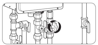
The water heater must be isolated from the gas piping system whenever the pressure testing will be less than and/or up to 1/2 psi (14 in. w.c. [3.5 kPa]). Closing the manual gas shut-off valve will isolate the water heater from the gas piping system.
