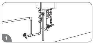
Install the manual gas appliance shut-off valve to the gas connection at the water heater. The shut-off is supplied with the water heater.
