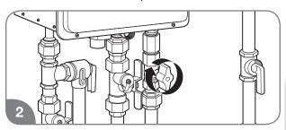
Turn the gas shut-off valve clockwise to the OFF position.
