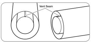
**NOTICE:** Make sure that the seam of the inner vent pipe in a horizontal run is towards the top of the installation as shown above.
