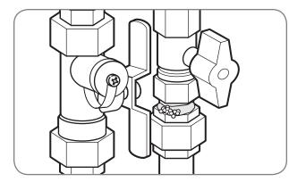
Turn on the gas shut-off valve(s) to the water heater.
