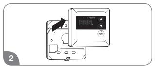
Remove the remote control from the base plate.
