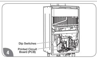
Find DIP Switch 1 located in the top-right portion of the PCB. The switch labeled "DIP 1" is the top switch.
