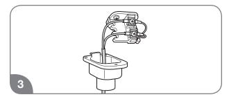
Connect the remote control extension cables from the remote control to the remote control connection terminals.
