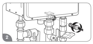
Reinstall the water filter in the base of the cold water inlet line.
