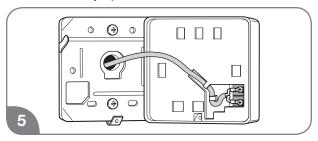
Connect the remote control to the remote control cable.
