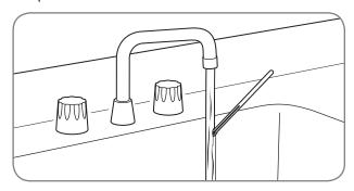
Turn on the hot water faucet and place a thermometer in the water stream.
