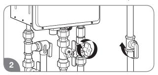
Close the gas shut-off valve(s).
