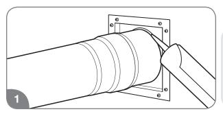
Apply high-temperature silicone sealant or silicone/latex caulk around the vent section. Completely seal where it passes through the wall plate and where it is attached to the structure. This will provide a weather seal for the system, so it must be a good seal.
