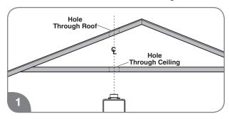
Cut a hole through the roof and interior ceiling to accommodate the vent pipe.
