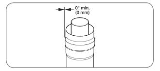
Minimum clearance around the coaxial vent pipe should meet the specifications listed on the instruction/warning label on the water heater. If no label is found, use the vent manufacturer's specifications or a minimum clearance of 0 in. (0 cm) around the vent pipe.
