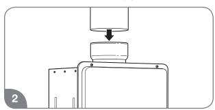
Complete the vent pipe installation to the water heater vent collar. If required, use high-temperature silicone sealant where the vent connector joins the water heater.
