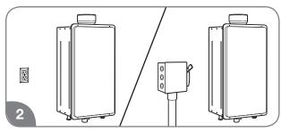
Make sure the proper electrical outlet or supply (120 VAC/60 Hz) is available and located near the unit. Direct-vent models come with a 6-ft. (1.8-m) power cord, while the outdoor models require hard-wiring or the addition of a plug.
