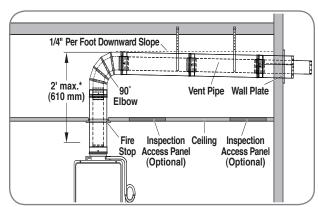
**ACAUTION:** The condensate collector must be used in horizontal terminations if vertical rise in the vent system exceeds 2 feet (610 mm).\*
