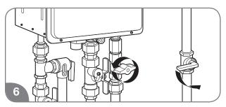
Open the gas shut-off valve(s).
