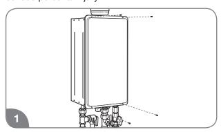
Remove 4 screws and the unit cover panel.
