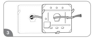
Feed the remote control cable through the large center hole in the base plate.
