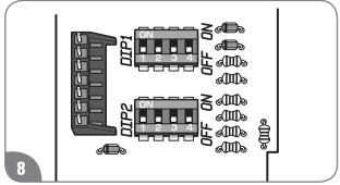
Change the fourth switch on "DIP 1" back to the OFF position (DOWN). The display of the remote control turns off.
