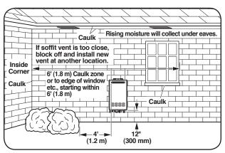
Install outdoor water heater such that air inlet and flue outlet are above anticipated snow level.
