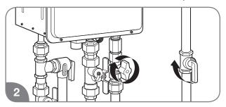
Close the gas shut-off valve(s).
