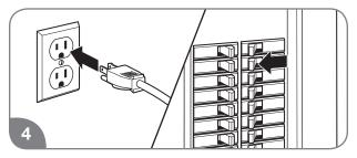
Turn on all electric power to the water heater. The water heater burner will automatically light when there is a demand for hot water.
