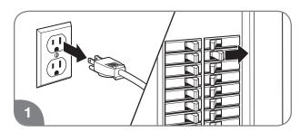
Disconnect all electric power to the water heater.
