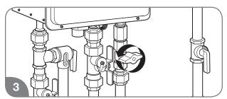
Turn the gas shut-off valve counterclockwise to the ON position.
