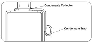
The drain tube is fashioned into a "pigtail" trap and must be filled with water to prevent flue gases from emitting into the building prior to operating the water heater.
