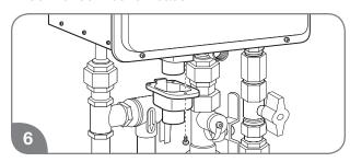
Reinstall the remote control connection cover and secure with the one screw.
