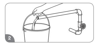
Before attaching the water line to the water heater, open the shut-off valve. Run the water until it has purged all contaminants (sand, debris, air, caulking).
