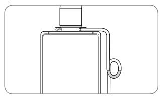
On a regular basis, inspect the condensate trap to ensure there is enough water in the trap and the condensate is draining properly.
