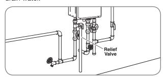
Annually check the operation of the pressurerelief valve. Lifting the lever handle on the pressure-relief valve opens the valve to flush hot water through the discharge line to the drain.
