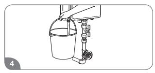
Open the drain valve in the COLD water outlet line to check the water flow through the water heater.
