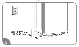
Position the water heater and tighten the adjustment screws to complete the installation. The rear of the water heater can be positioned anywhere between 3/8 in. (0.95 cm) and 1 1/2 in. (3.8 cm) from the wall (indoor model only).
