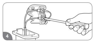
Firmly tighten the terminal screws by hand.
