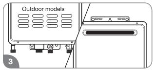
Check the air intake and vent outlet for blockage and/or debris.
