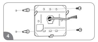
Install the base plate to the wall using suitable screws and wall anchors.
