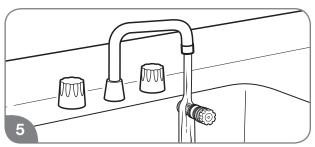
Clean the water filter under running water. To remove severe sediment and dirt, use a soft brush.
