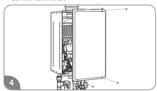
Turn off the hot water faucet and reinstall the unit cover panel.
