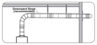
When a water heater is **vented horizontally**, the vent pipe should have a DOWNWARD or UPWARD slope towards the termination. If an UPWARD slope is used, always attach a drain hose to the condensate collector and plumb the hose to a sanitary sewer drain.
