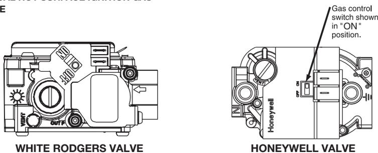
6. Turn manual gas control knob clockwise or set the gas control switch to the "OFF" position. See Figure 5.
