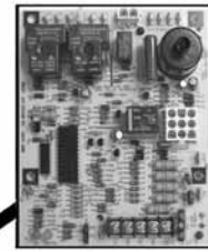
INTEGRATED FURNACE CONTROL
