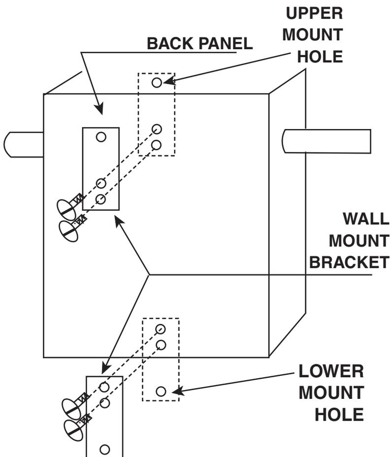
Mounting kit contains sheet metal screws and supporting brackets in a plastic bag.
