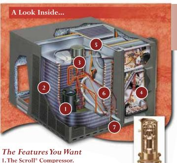
All of our residential package units - regardless of efficiency level — feature the Scroll® Compressor. The scroll compressors uses a more advanced technology than traditional reciprocating compressors. They have fewer moving parts, and they are quieter, more efficient, and longer lasting.
