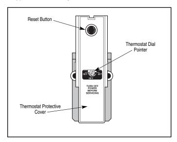
The illustration above shows the temperature adjustment dial used for setting the water temperature. Refer to Operation section of this manual for detailed instructions in how to adjust the thermostat.
