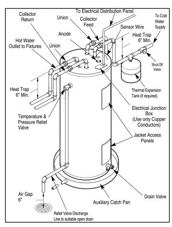
Figure 2.—Typical Installation for Top Connect Models
