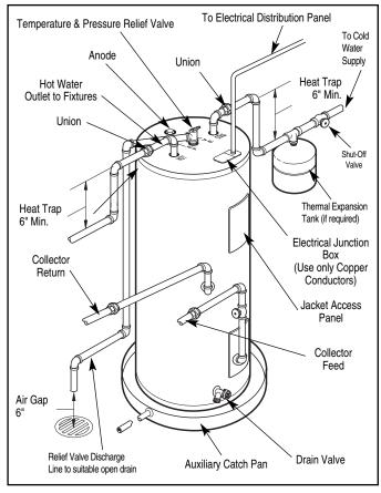
Figure 2.—Typical Installation for Side Connect Models
