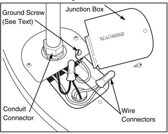
Figure 3. — Water Heater Junction Box.
