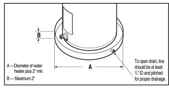
Figure 1. — Auxiliary Catch Pan
