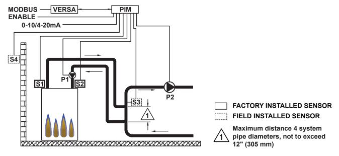
Figure 13. MODE 1 - Single Boiler with Primary/Secondary Piping
