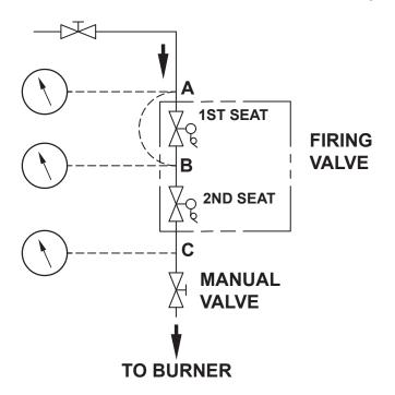
Figure 45. Leak Test Procedure
