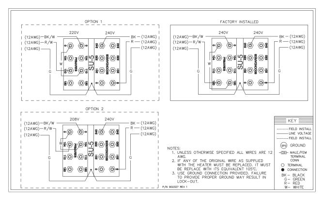
Figure 21. Wiring Diagram Transformer 240V (Factory Installed) and 208V/220V (Field Wiring)
