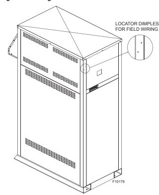
Figure 23. Locator Dimples for Optional Components
