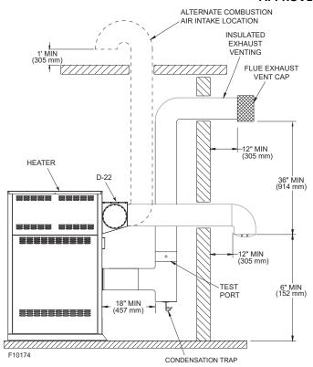
Figure 31. Horizontal Through-the-Wall Direct Venting
