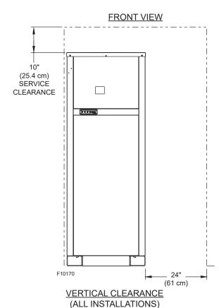
Figure 6. Minimum Clearances from Combustible Surfaces – Indoor or Outdoor Installations
