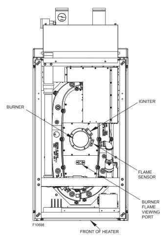
Figure 4. Component Locations - Top View
