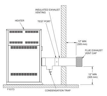
Figure 30. Alt. Horizontal Through-the-Wall Venting
