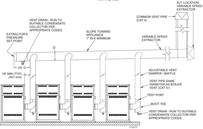
Figure 28. Typical Common Venting
