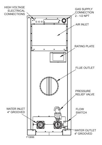
Figure 3. Component Locations - Rear View
