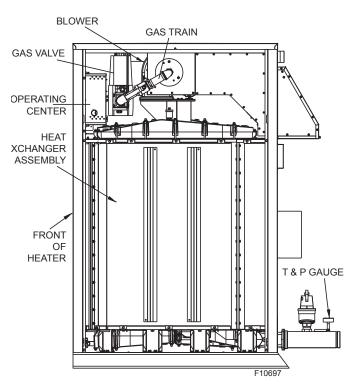
Figure 2. Component Locations - Side View
