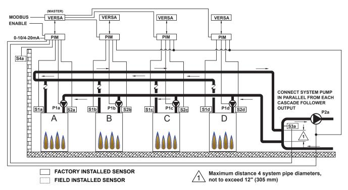
Figure 15. MODE 1 - Recommended Boiler Cascade with Primary/Secondary Piping
