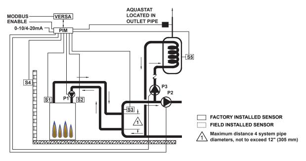
Figure 14. MODE 2 - Single Boiler with Indirect on System Loop - Primary/Secondary Piping
