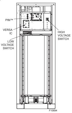
Figure 1. Component Locations - Front View
