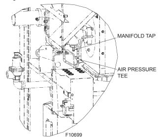
Figure 43. Air Pressure Tee
