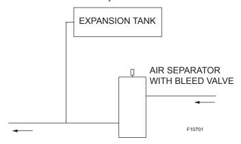
Figure 12. Air-Separation/Expansion Tank
