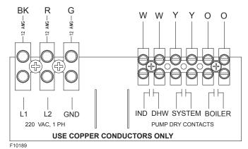
Figure 24. MVB Cascade Master Pumps
