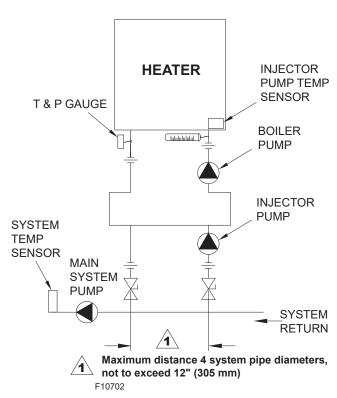
Figure 11. Cold Water Run
