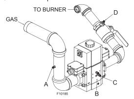
Figure 42. Gas Pressure Measurement Locations
