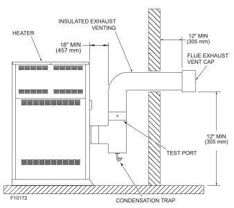
Figure 29. Horizontal Through-the-Wall Venting
