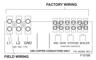
Figure 19. Wiring Electrical Connections
