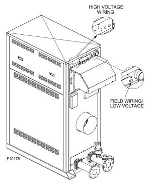
Figure 22. Wiring Location
