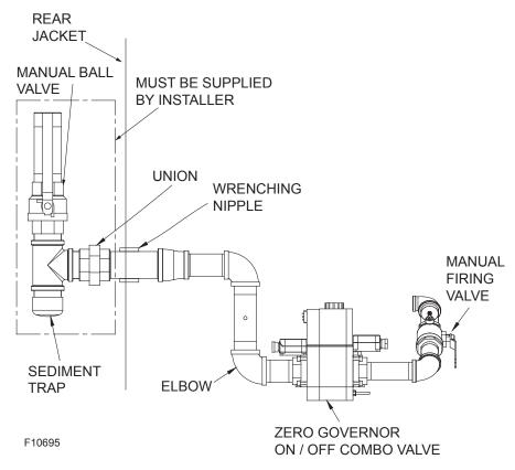
Figure 18. Gas Supply Connection
