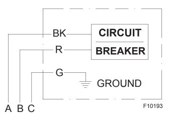
Figure 20. Wiring Connections
