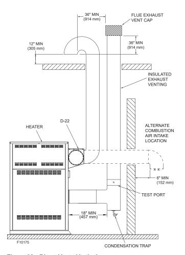
Figure 32. Direct Vent - Vertical
