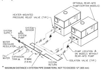
Figure 19. Dual Heaters (Reverse/Return) with Primary/ Secondary Piping
