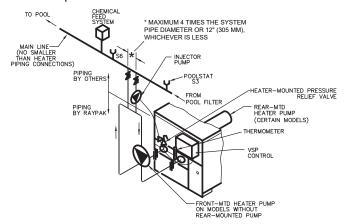
Figure 26. Single Pool Heater - Automatic Bypass
