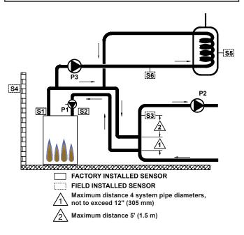
Figure 21. MODE 3 - Single Boiler with Indirect on Boiler Loop
