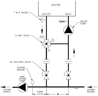
\* MAXIMUM DISTANCE 4 SYSTEM PIPE DIAMETERS, NOT TO EXCEED 12" (305 mm).
