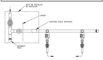
Figure 27. Gas Supply Connection
