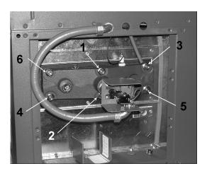
Figure 8. Torque Sequence
