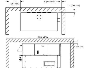
Figure 6. Minimum Clearances from Combustible Surfaces – Indoor Installations
