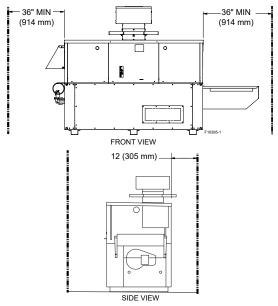
Figure 7. Minimum Clearances from Combustible Surfaces – Outdoor Installations
