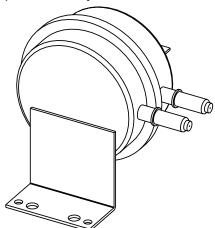
Figure 47. Blocked Vent Switch
