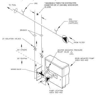
Figure 24. Single Pool Heater Application
