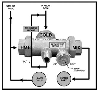
Figure 25. Mixing Valve Configuration
