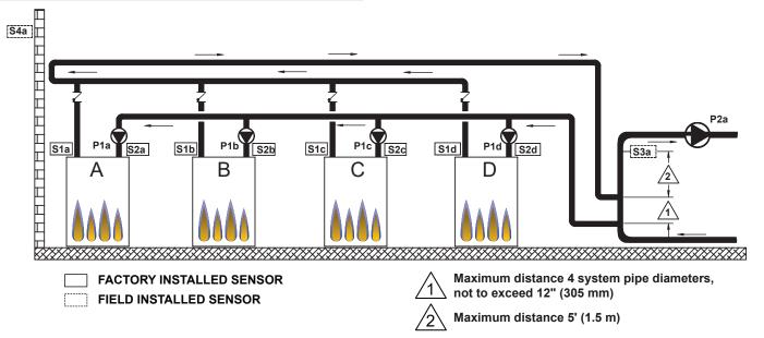
Figure 18. MODE 1 - Boiler Cascade with Primary/Secondary Piping
