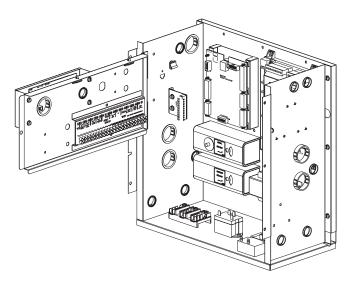
Figure 32. Low Voltage Field Wiring Location
