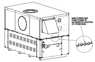
Figure 31. Wiring Location
