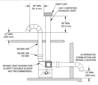
Figure 40. Ducted Air - Vertical
