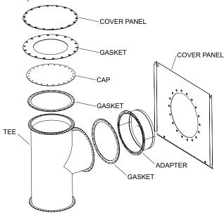
Figure 35. D-14 Flue Exhaust Tee Kit
