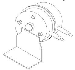
Figure 46. Air Pressure Switch
