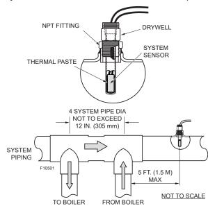
Figure 15. System Sensor Installation
