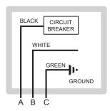
Figure 29. Wiring Connections
