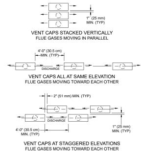
Figure 39. Vent Cap Configurations
