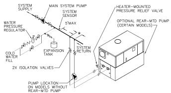
\* MAXIMUM DISTANCE 4 SYSTEM PIPE DIAMETERS, NOT TO EXCEED 12" (305 mm).
