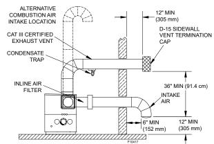
NOTE: WHEN VERTICAL HEIGHT EXCEEDS 25 FT (7.62 m), CONSULT FACTORY PRIOR TO INSTALLATION.
