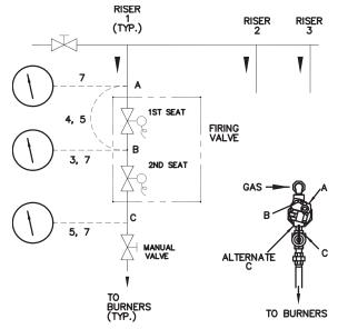
Figure 50. Leak Test
