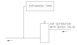
Figure 14. Air-Separation/Expansion Tank
