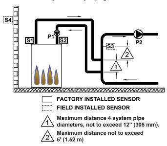
Figure 17. MODE 1 - Single Boiler with Primary/Secondary Piping
