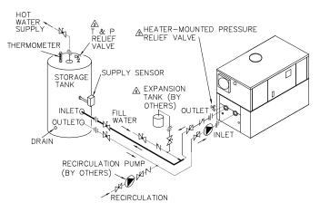
Figure 22. Single Domestic Hot Water Heater and Storage Tank
