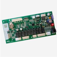
**MICROPROCESSOR** control is more precise than mechanical systems. It controls temperatures to within a half degree of the desired set point. Service technicians can easily view the service history of the unit.
