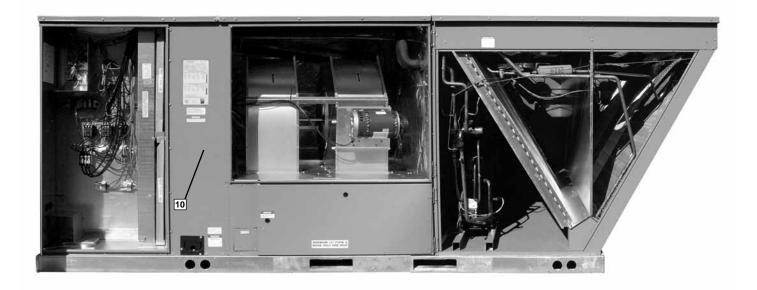
A control box component location legend sticker (11) is located on the left interior surface of the control section to match the components to the wiring diagram for ease of trouble shooting. Wiring is numbered on each end of the termination and color-coded to match the wiring diagram. The control transformer has a low voltage circuit breaker that trips if a low voltage electrical short occurs. There is a blower contactor and contactor for each compressor.
