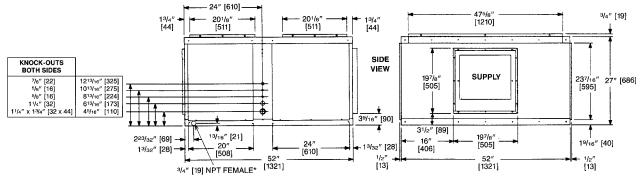
\*Drain connections are provided on both sides of the drain pan. The drain can be connected to either side of the drain pan, but not both. The drain must be trapped.
