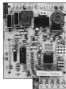
INTEGRATED FURNACE CONTROL
