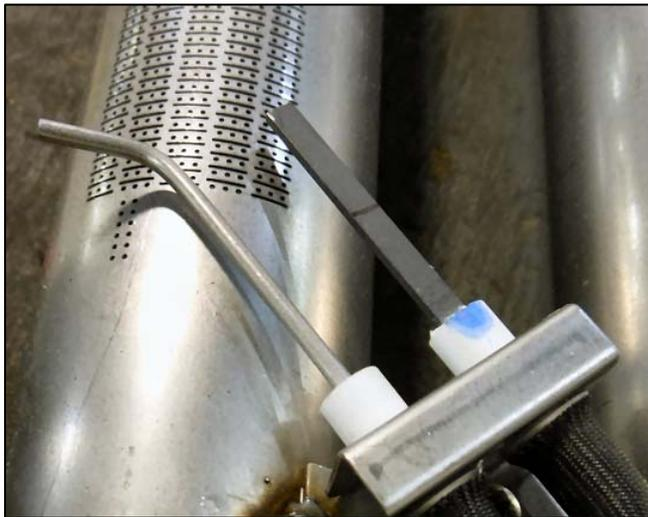
Hot surface igniter should extend over closest row of burner tube holes.
