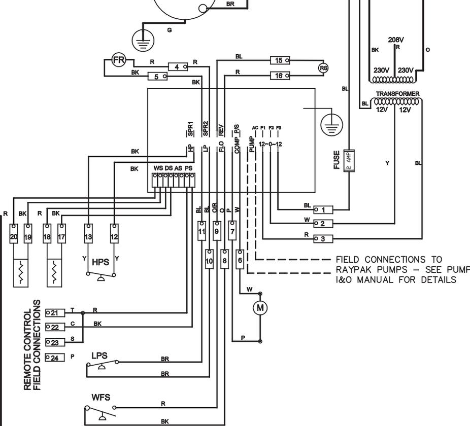
3. FOR 2 WIRE REMOTE CONTROL: USE TERMINALS 21 & 22 TO ATTACH 2 WIRE CONTROL SYSTEMS THAT HAVE THEIR OWN SENSORS FOR TEMPERATURE CONTROL. SET POOL TEMPERATURE TO OFF AND SPA TEMPERATURE TO 104°.
