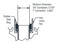
The hot water connection fitting must have a inside diameter greater than the minimum shown in the picture above.
