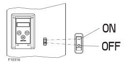
Figure 44. Heater Toggle Switch
