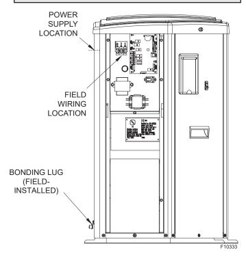
Figure 20. Wiring Locations
