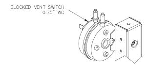
Figure 40. Blocked Vent Switch
