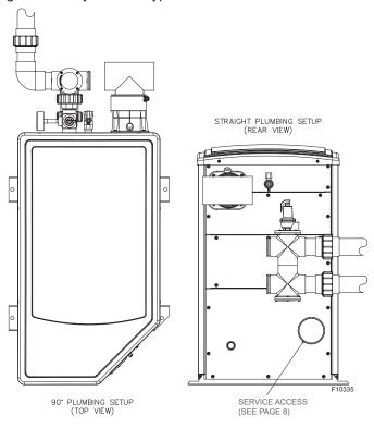
Figure 23. Plumbing Setup
