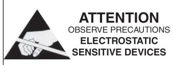
NOTE: Electrostatic Discharge (ESD) damage can be caused by direct or indirect contact with the wiring or circuit board. When one walks to the heater area, an electrostatic charge accumulates on the body. Contact of a finger allows the body to discharge, possibly causing device damage. This damage can be limited if the service person discharges himself, following ESD preventive/ removal practices, and holds on to the heater enclosure for 5 seconds before proceeding.
