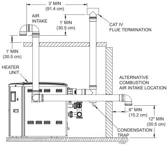
Figure 11. Direct Vent - Vertical
