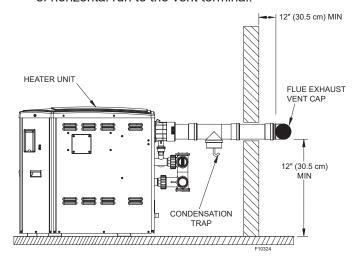
Figure 8. Horizontal Through-the-Wall Venting
