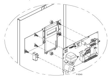
Figure 30. Removing the Ignition Control Board
