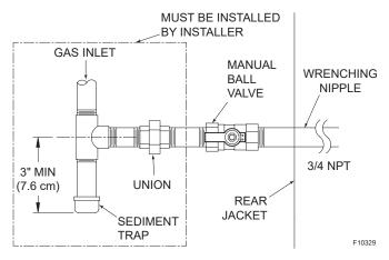
Figure 15. Gas Supply Connections
