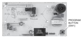
Figure 31. Ignition Control Board
