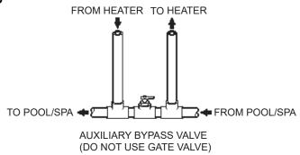
Figure 18. Auxiliary Bypass Valve
