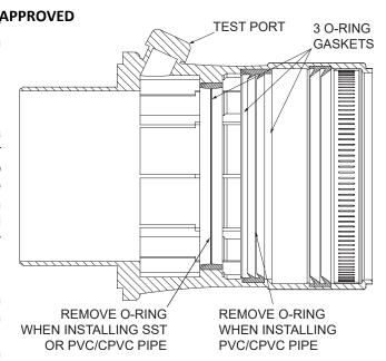
Figure 13. Multi-Vent Adapter
