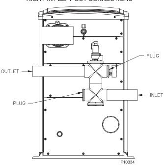
Figure 22. Water Connection Configurations
