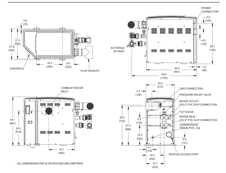
Figure 3. Specifications and Dimensions
