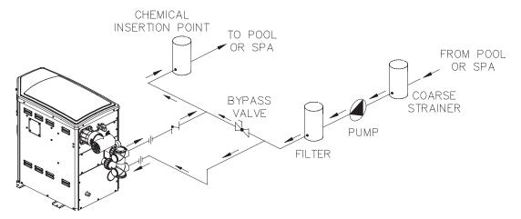
Figure 24. Single Pool or Spa Heater Installation
