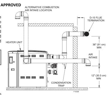
Figure 9. Horizontal Through-the-Wall Direct Venting
