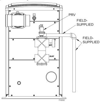
Figure 19. PRV Piping
