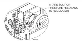
Figure 45. Air Intake Pressure Measurement Location
