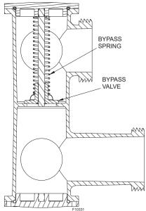
Figure 17. External Automatic Bypass Valve
