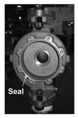
Fig. 37: Be sure not to damage the seal when removing or replacing the pump body
