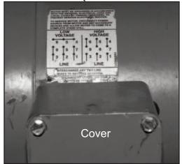
Fig. 32: Pump Wiring Decal and Junction Box
