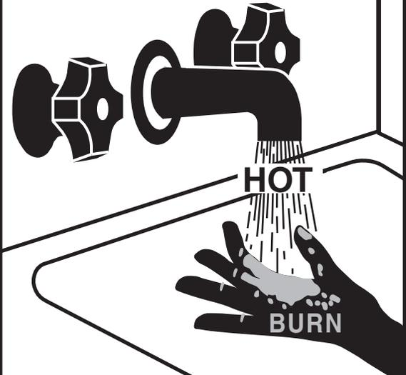
**Water temperature over 125°F can cause severe burns instantly or death from scalds.**
