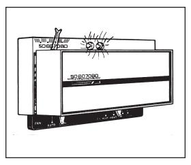
Lights may be used to indicate that the auxiliary electric heat is operating. The lights may be different colors on different types of thermostats. Typical lights will be blue or green for normal auxiliary heating and red for emergency heat.
