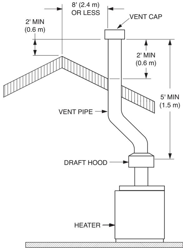
Figure 11. Venting Clearances
