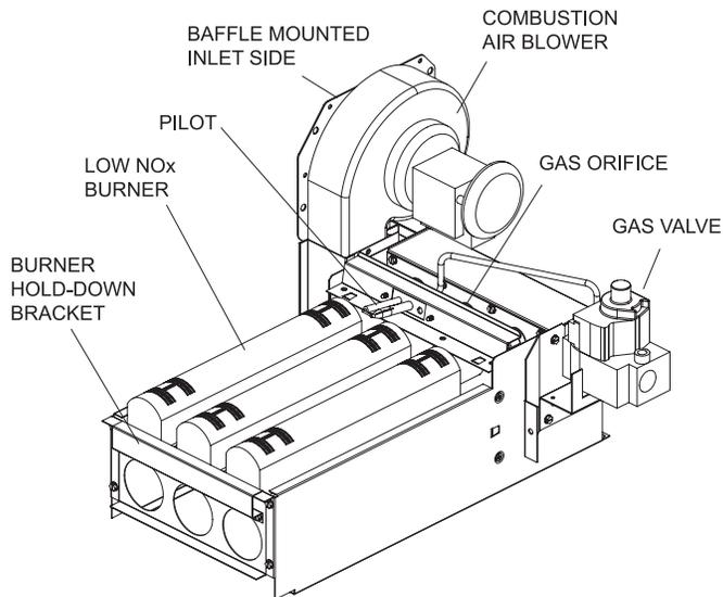
Figure 54. Burner Tray Assembly
