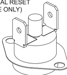
Figure 53. High Limit Switches
