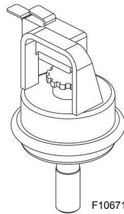
Figure 50. Water Pressure Switch Assembly
