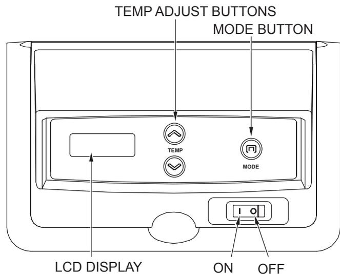
Figure 37. Control Adjustments
