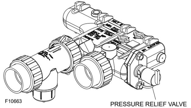
**Figure 25. Pressure Relief Valve Bronze Header (ASME Models)**
