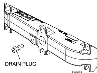
**Figure 63. Return Header Drain Valve, Bronze ("B" Prefix Models)**
