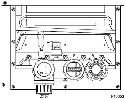
**Figure 27. Component Wiring Locations - In/Out Header**
