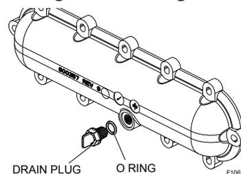
**Figure 62. Return Header Drain Plug, Polymer ("P" Prefix Model)**
