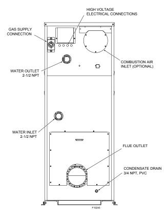
Figure 3. Component Locations - Rear View
