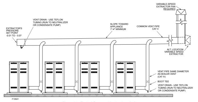
Figure 38. Typical Common Venting Installation
