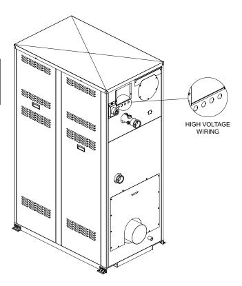
Figure 27. Wiring Location - High Voltage
