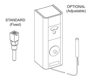
Figure 43. High Limit (Manual-Reset)
