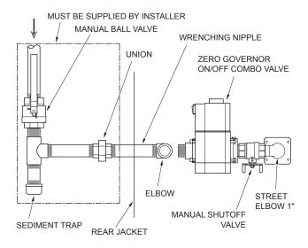
Figure 23. Gas Supply Connection
