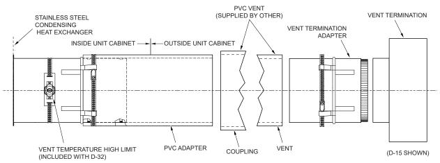
Figure 41. D-32 PVC Vent Adapter
