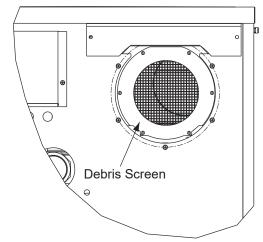
Figure 11. Remove the Debris Screen
