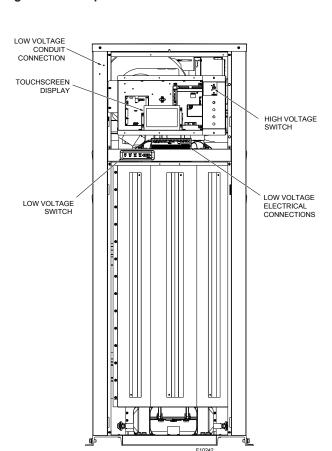
Figure 2. Component Locations - Front View
