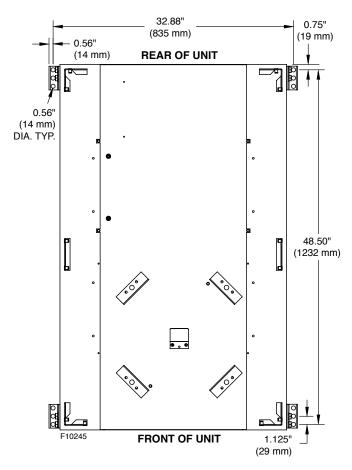
Figure 5. XTherm 1005A-2005A Anchor Hole Locations
