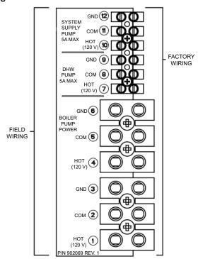
Figure 24. Wiring Electrical Connections
