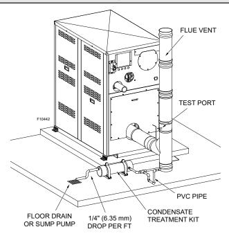
Figure 40. Visual Guide for Condensate Piping
