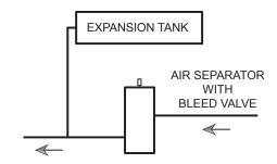
Figure 14. Air-Separation/Expansion Tank
