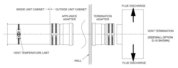
Figure 42. D-33 Centrotherm Polypropylene Vent Adapter
