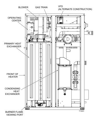
Figure 1. Component Locations - Side View
