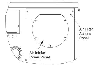
Figure 10. Remove the Air Intake Cover
