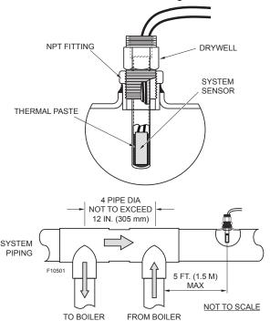
Figure 13. System Sensor Installation
