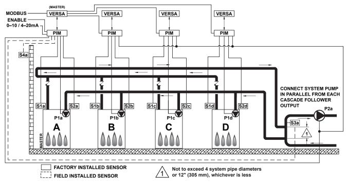
Figure 17. Mode 1 - Boiler Cascade with Primary/Secondary Piping
