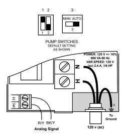
Figure 45. Injector Pump DIP Switches, and Wiring
