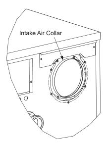
Figure 12. Install the Intake Air Collar
