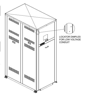
Figure 28. Locator Dimples for Low-Voltage Conduit
