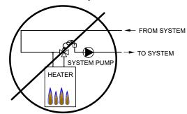
Figure 15. Three-Way Valves (Usage as shown NOT supported)
