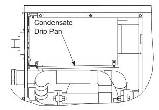
Figure 9. Install the Condensate Drip Pan
