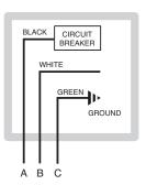
Figure 25. Wiring Connections
