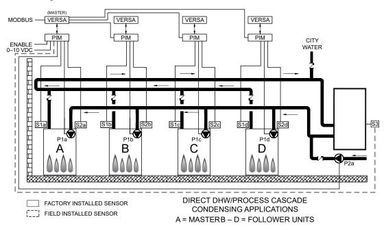
Figure 21. WH Units – Water Heater Cascade with Tank H Units - Boiler Cascade with Process Tank
