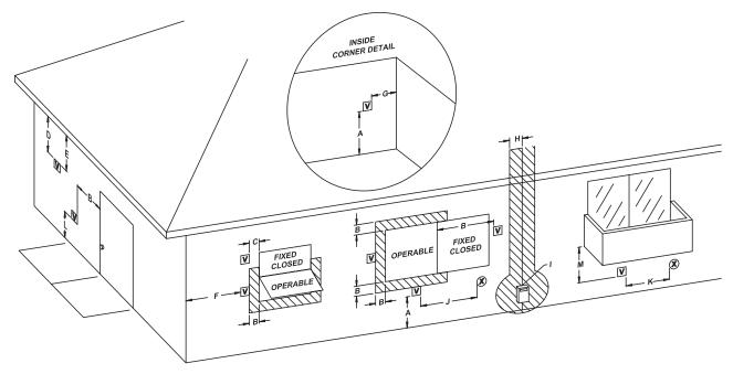
Figure 7. Minimum Clearances from Vent/Air Inlet Terminations – Indoor and Outdoor Installations
