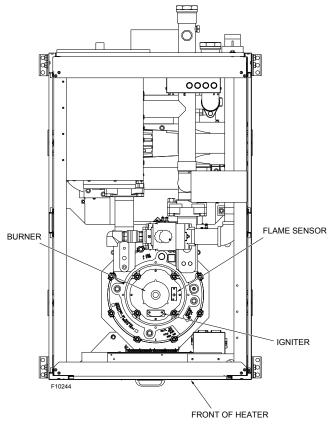
Figure 4. Component Locations - Top View
