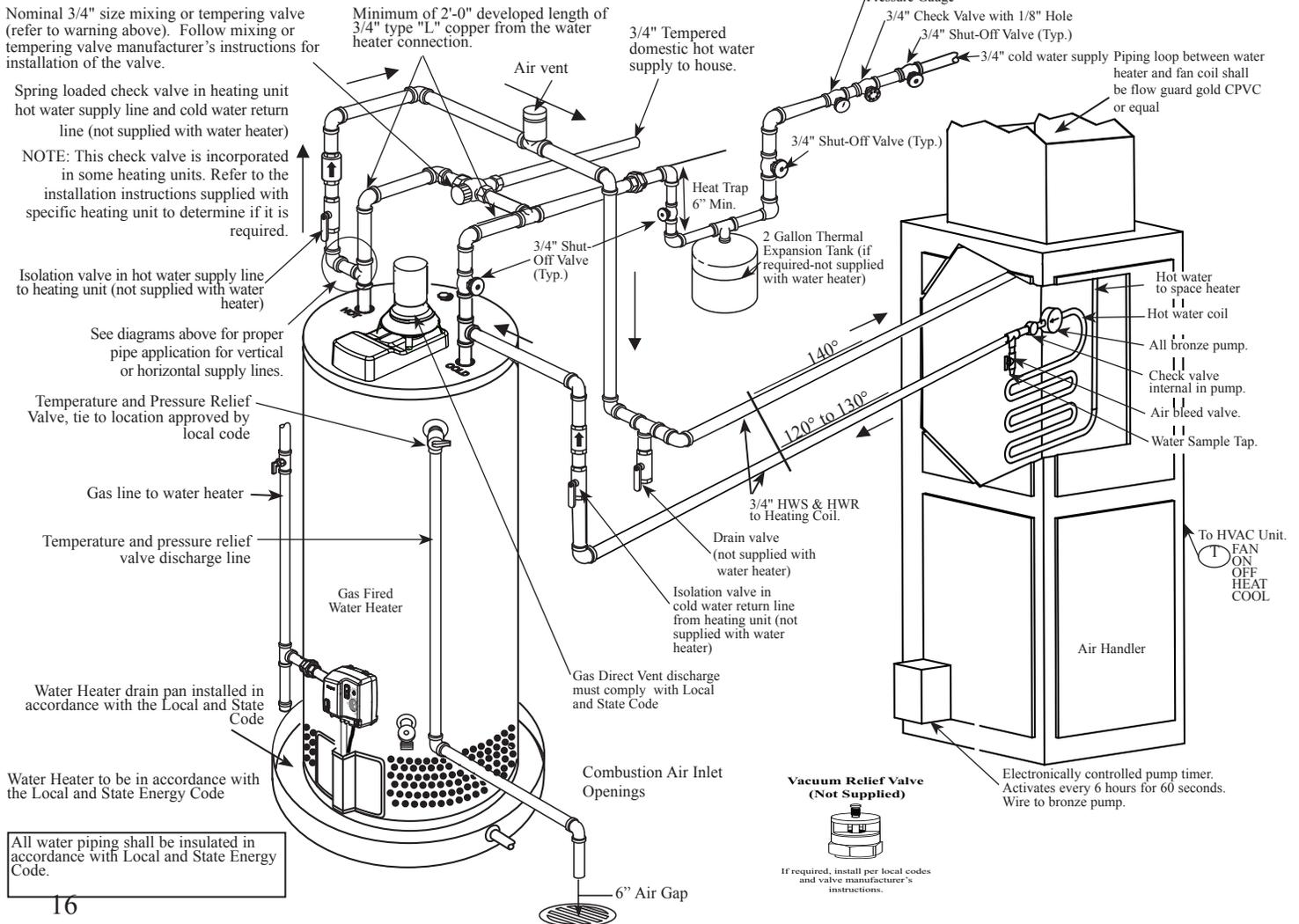
All water piping shall be insulated in accordance with Local and State Energy Code.
