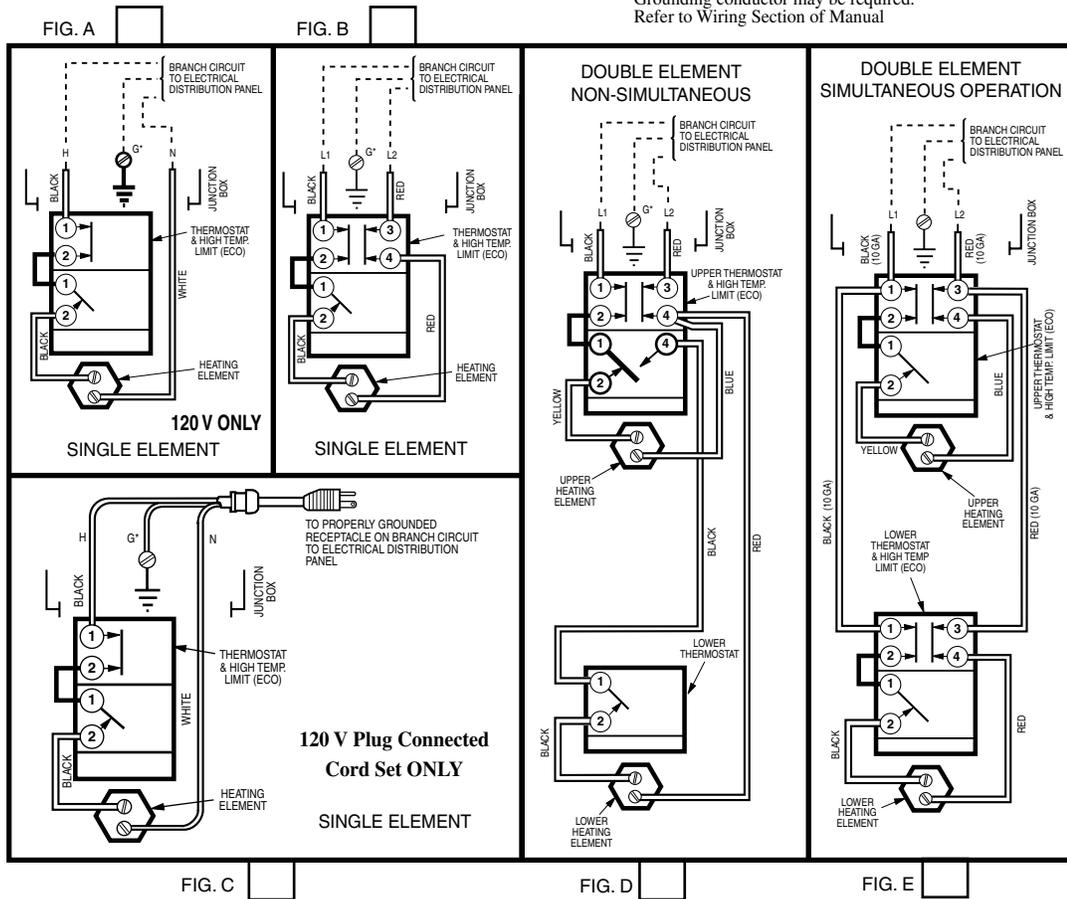
**THIS ELECTRIC WATER HEATER IS WIRED AS INDICATED ABOVE**
