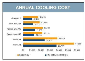
Pacific Northwest National Laboratory (PNNL) Rooftop Comparison Calculator Assumptions: Equipment Comparison: 10 ton 12.5 EER Variable Frequency supply fan compared to a 9 EER constant volume supply fan; Building Type: Retail Stand Alone; Schedule: All Week 6 a.m. to 10 p.m.; Electrical Cost: 11.5 cents/kWhr; Equipment Life: 15 Years.
