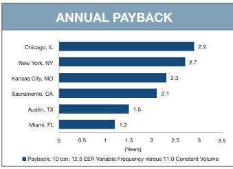
Pacific Northwest National Laboratory (PNNL) Rooftop Comparison Calculator Assumptions: Equipment Comparison: 10 ton 12.5 EER Variable Frequency supply fan compared to a 11 EER constant volume supply fan; Building Type: Retail Stand Alone; Schedule: All Week 6 a.m. to 10 p.m.; Electrical Cost: 11.5 cents/kWhr; Equipment Life: 15 Years.
